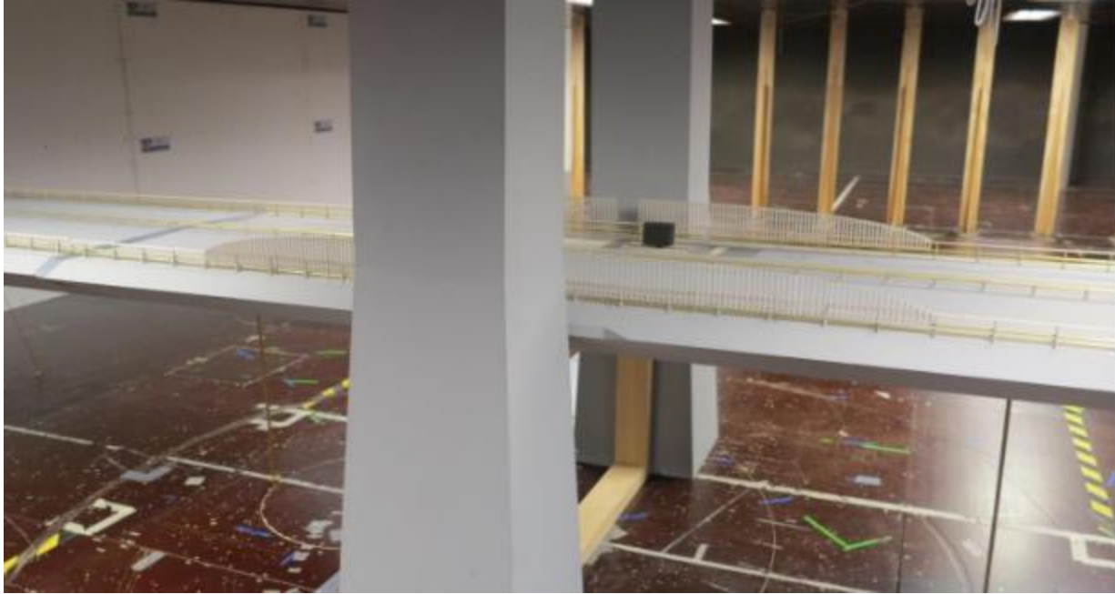
Figure 1. 1:30 scale model of the Storebælt tower deck assembly carrying local wind screens and model of auto-trailer.
